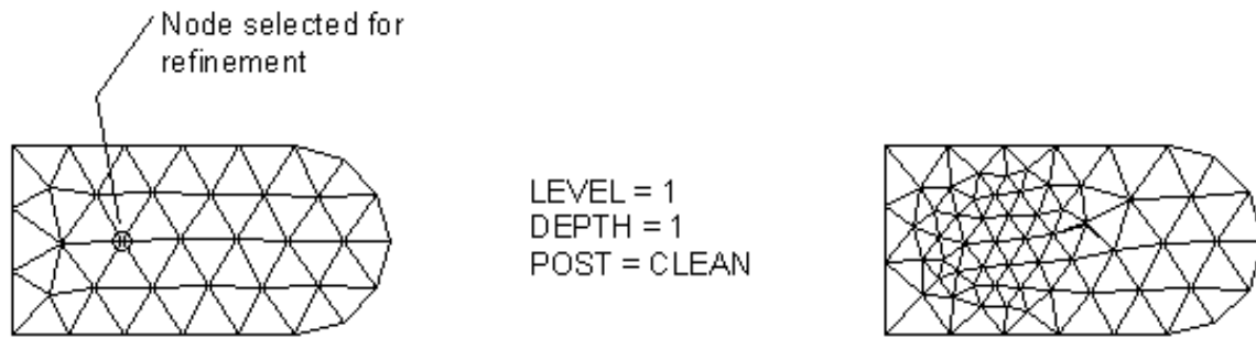
(a) Mesh refinement around a node [ NREFINE ]
