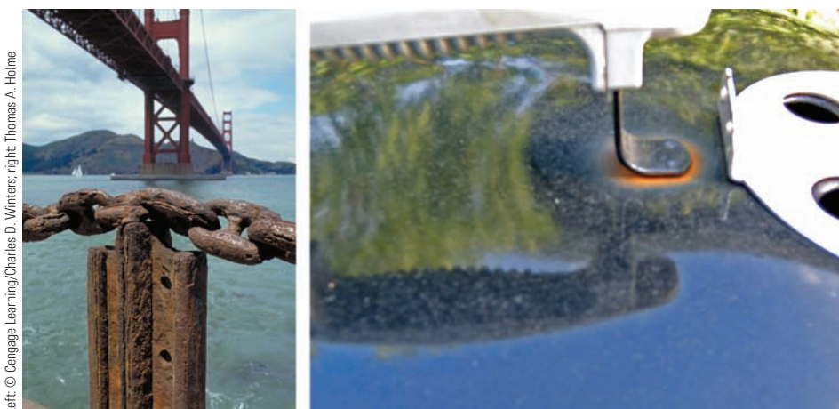
Figure 13.1 ■ Corrosion occurs in a variety of forms. The chain on the left shows uniform corrosion, whereas the grill cover on the right shows corrosion only where the handle is attached. This is called crevice corrosion and can occur whenever small gaps exist between metal parts.
