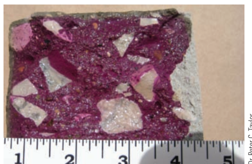
Figure 12.2 ■ Treatment of concrete with phenolphthalein reveals the chemical effects of weathering. The pink color shows that the bulk of this sample remains basic, even after extended exposure to the elements. The colorless area at the top, which is the surface that was actually exposed, is no longer basic. Reaction with atmospheric \text{CO}_2 has neutralized the hydroxide in this surface region.
