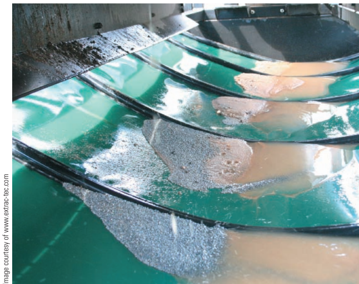
Figure 3.10 ■ Gravity separators like this one from Extrac-tec are used in remediation of lead from firing ranges. Differences in density and solubility allow the equipment to extract lead or other heavy metals from soil.
