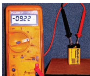
Figure 13.7 ■ An electric potential has a fixed polarity and voltage. Reversing the poles of a battery with respect to a voltmeter changes the sign on the measured voltage but does not actually influence the electrochemical reaction in the battery.
