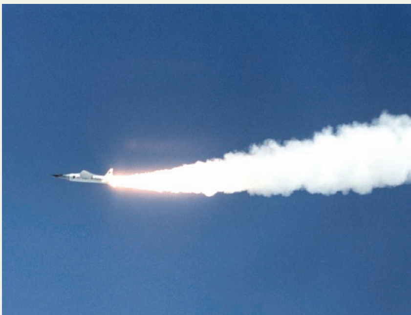
Chemical reactions initiated in the Pegasus rocket accelerate NASA's X-43A aircraft to hypersonic speeds. In a test flight, the X-43A approached Mach 10, ten times the speed of sound. NASA Dryden Flight Research Center
