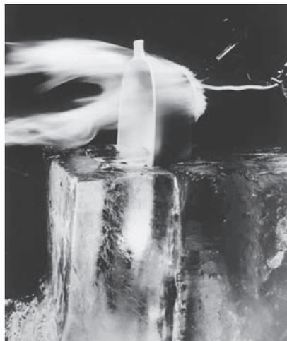
**FIGURE 11.2** Cookware made of a glass-ceramic provides good mechanical and thermal properties. The casserole dish can withstand the thermal shock of simultaneous high temperature (the torch flame) and low temperature (the block of ice). (Courtesy of Corning Glass Works.)
