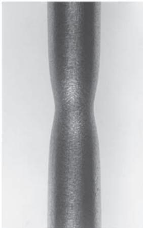
**FIGURE 6.7** Neck down of a tensile test specimen within its gage length after extension beyond the tensile strength. (Courtesy of R. S. Wortman.)
