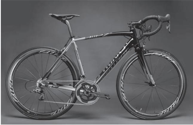
This elegant road bike uses a carbon-fiber reinforced polymer composite to provide optimal performance. (© Hugh Threlfall / Alamy.)
