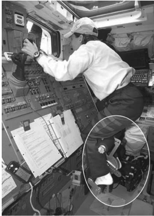
Figure 7 Operating the remote manipulator system requires a stable restraint carefully adjusted.
