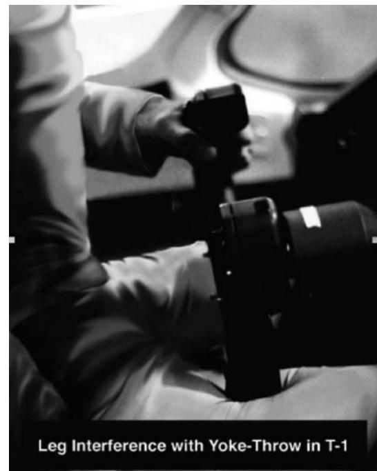
Figure 2 Problem that occurred when using 1st percentile female and 99th percentile male.
