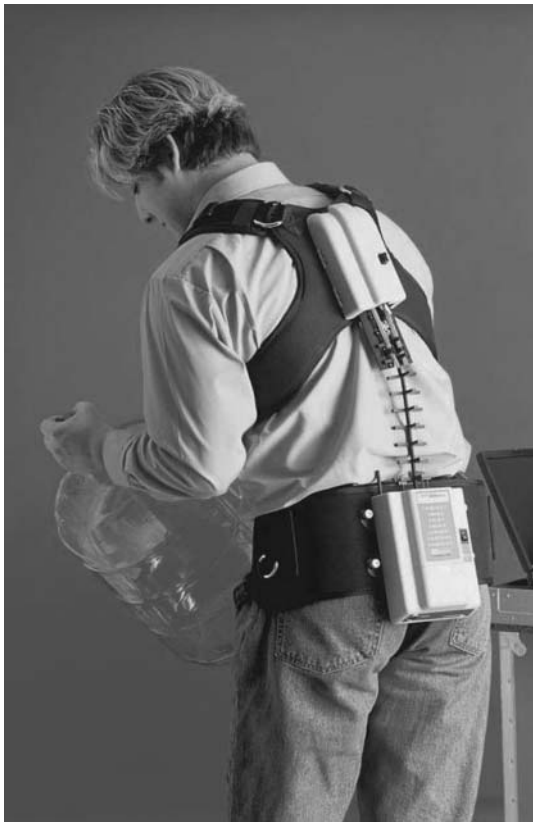
Figure 9 LMM used to track trunk kinematics during occupational activities.
