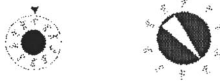
Figure 12 The design of a knob can greatly affect its usability by people with low vision or blindness.
