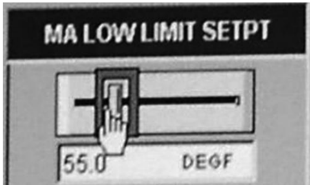
FIGURE 7.11 Virtual slideswitch emulates a real-world control.
