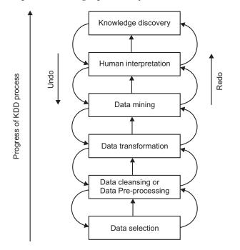
FIGURE 13.5. Data mining process (KDD).
