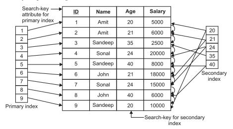
FIGURE 3.21. Primary and secondary index.
