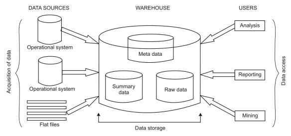
FIGURE 13.1. Data warehouse architecture.
