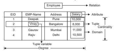
FIGURE 4.22. Basic data structures of relational database.
