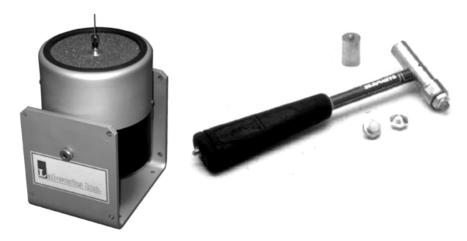
FIGURE 11.3 Modal test inertial shaker, inertial hammer, and accelerometer.
