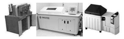
**FIGURE 11.16** Industrial oven, salt spray chamber, and corrosion test chamber.
