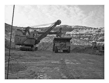
**FIGURE 9.9** Haul truck being loaded by excavator.
