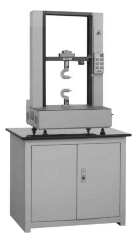
**FIGURE 6.7** Universal strength of materials test machine.
