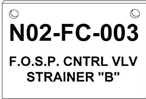
Figure K.4 Example of 2 3/8-inch equipment tag for North Station Unit no. 2 Fuel Oil Service Pump Control Valve Strainer B.
